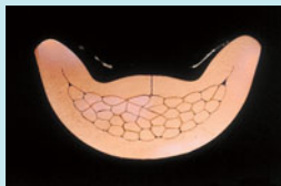
Cross section of crimping of stranded wire
