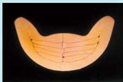
Cross section of crimping of flat wire
