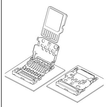
This is micro SD card cnnector of flip cover type that can approach from above the PC board surface.
