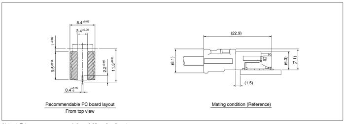
Note: 1. Tolerances are non-cumulative: ±0.05mm for all centers. 2. The dimentions above should serve as guideline. Contact JST for details.
