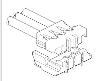
This ADH connector is compact and low profile type, height 1.9mm and width 4.3mm, 1.3mm pitch wire-to-board connector.
