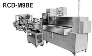
Auto. ID machines for 2.5 mm & 2.0 mm pitch jumper wires
