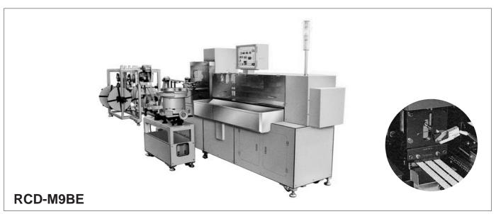
This automatic machine processes 2.0mm and 2.5mm pitch jumper wires, including cutting to predetermined length, slotting, semi- or full-stripping and kinking. It also simultaneously fits insulation displacement connectors to one or both ends of the cable.
