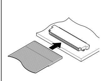
The large miniaturization at pitch direction and depth direction and low profile as 1.2mm mounting height are realized. FH connector is miniaturized and space saving Non-ZIF type connector for FPC.
