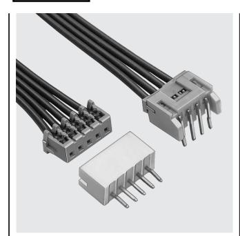
The CR 2.0mm insulation displacement connector features a mounting height as low as 6.9mm and a thickness as thin as 4.8mm (for top entry type). It's suitable for interconnection of UL1007 electric wires in a wide range of electrical and electronic equipment such as VCRs and video cameras.
