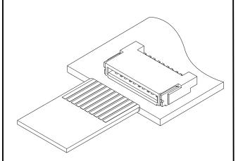
This is a 0.4 mm pitch, compact Non-ZIF type connector with a mounting height of 1.0 mm and a depth of 3.0 mm.
