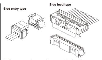
This connector can be mounted on the same PC board layout as GH connector, and has the sucking area on the top of connector without suction tape. The side feed type for drawing out the wire laterally that considers the workability of mating and normal side entry type has been developed.
