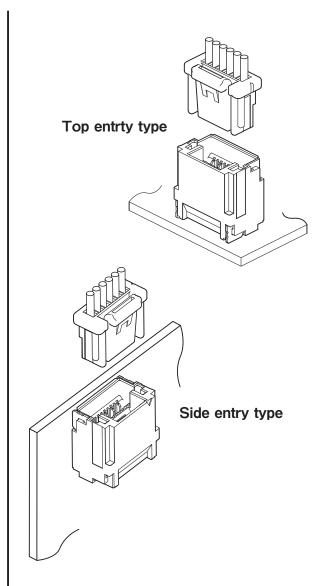
This is a 1.0 mm pitch, wire-to-board, SMT connector designed for ingress protection against potting material on the PCB. This potting-compatible version of the NSH connector features a strong locking function and delivers a noticeable click feeling during insertion. Together with low-insertion force contacts, the NSH connector facilitates a reliable mating operation.
