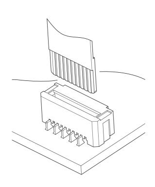
This is low profile 0.4mm pitch Non-ZIF top entry type connector with a mounting height of 2.5mm.
