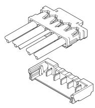
This AUH connector is compact and low profile type, height 1.85mm and width 5.2mm, wire-to-board connector. And also 5A in rating current was realized.
