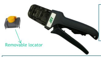
Maintain the pushed locator, insert the contact, release then place the bare thread.
