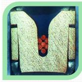
An *Insulation Displacement Connector* (*IDC*) which is also known as *Insulation Piercing Contact* (*IPC*), is an electrical connector designed to be connected to the conductor of an insulated cable by a connection process which forces a selectively sharpened blade through the insulation, bypassing the need to strip the insulation conductors before connecting.
